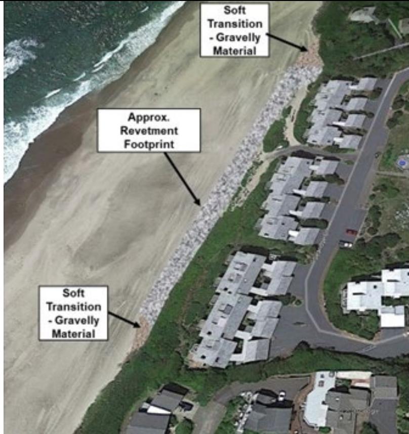
Conceptual plan view of armor rock revetment at Searidge Condominiums; footprint approximately 35,000 square feet.
