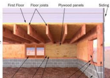
Figure A. Strengthening weak crawlspace walls.
